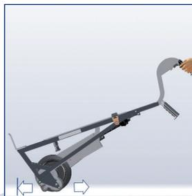
Test: CargoMaster cannot be pushed forward, only backward.
