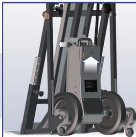
Pull out the lockin pin (only A350) and remove battery pack.
