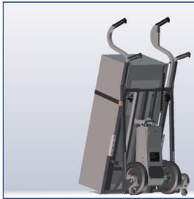
Secure load with lashing strap.
