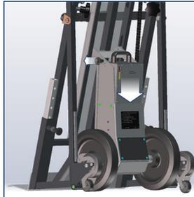
Pull out the lockin pin (only A350) and reattach battery pack.
